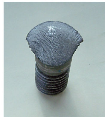
Fig. 3 — Hydrogen embrittlement and failure of a hard chromium-plated chain conveyor bolt.
